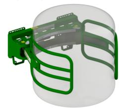
When stacking bales, either of the two paddles can be locked in position, allowing the other to do all the movement. This feature, along with the slimline, robust tube used in the paddles, ensures the bales can be stacked tightly together without compromising the bale integrity.
